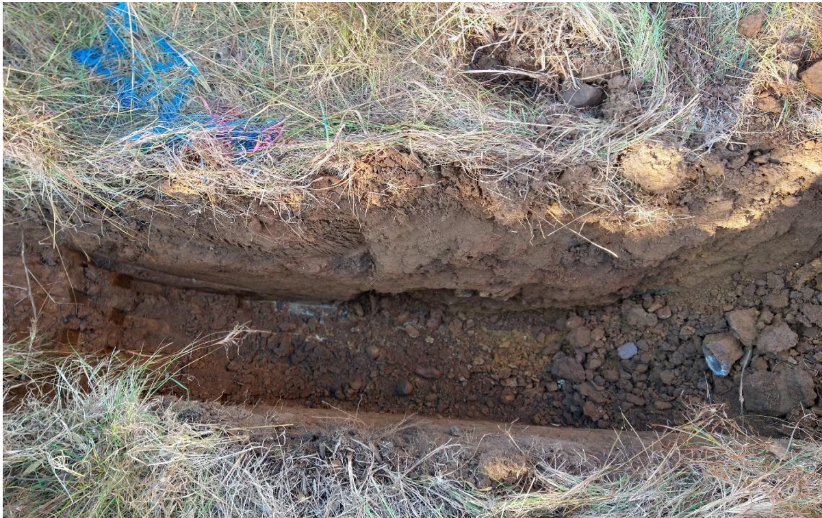
Photo 9: Test Pit 123 showing profile where the Luddenham Dyke was encountered (Refusal at 0.9m)
