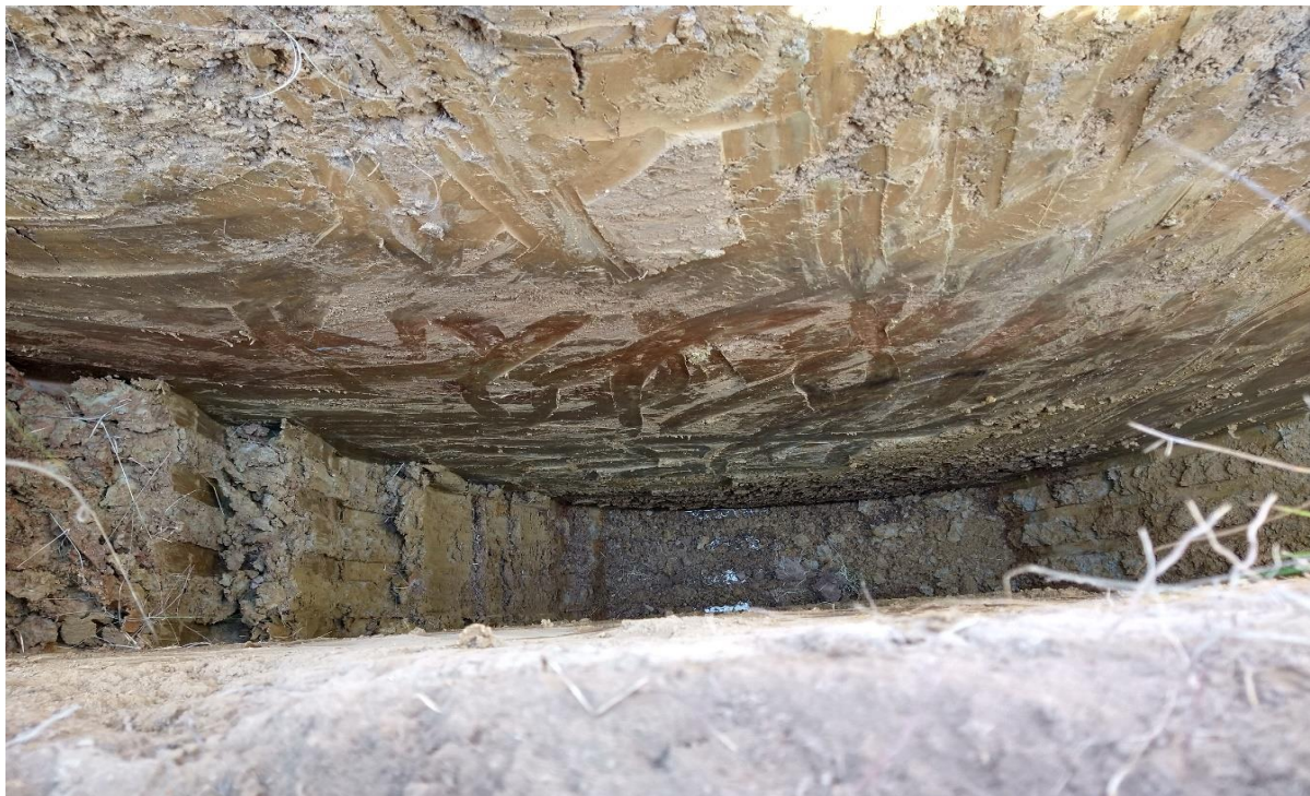
Photo 11: Test Pit 205 in stormwater corridor showing typical alluvial soil profile
